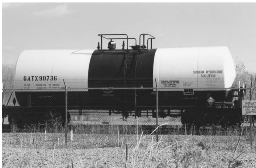
Tank car of sodium hydroxide solution, a corrosive material.
