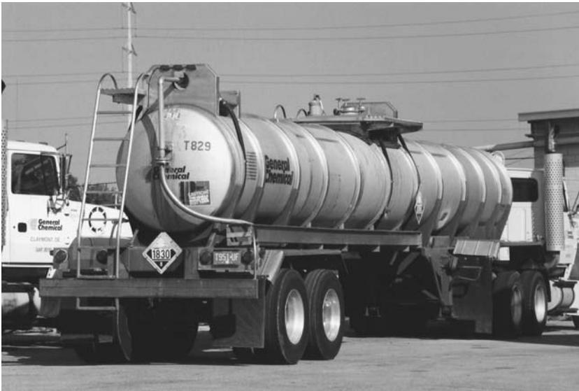
MC/DOT 312/412 tanker for heavy corrosive materials.
